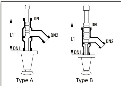
These valves prevent the accumulation of solids or liquid in the bottom outlet of a vessel. This valve can be incorporated in any spherical or cylindrical vessel.
