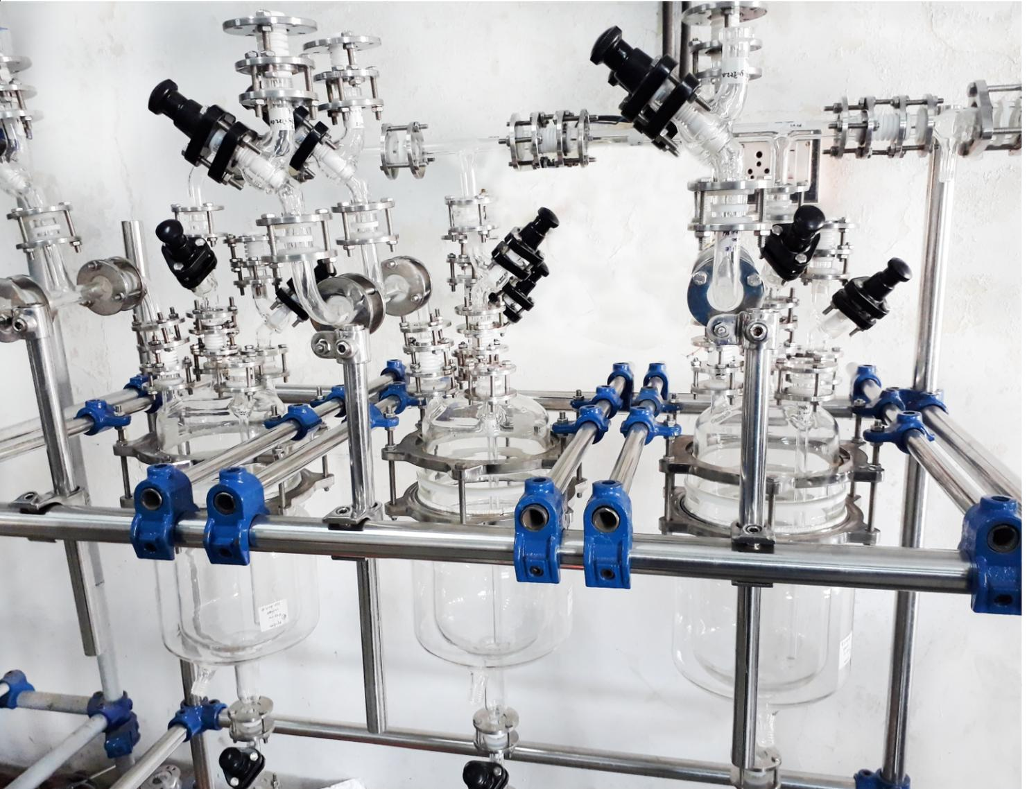
A wide variety of valves are described in this section. All the valves are made of Borosilicate Glass body & PTFE plug so that process fluid just comes in contact with Glass & PTFE only. Borosilicate Glass body permits the visual checking of the operation.
