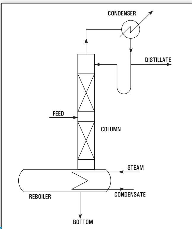
The limitations of batch distillations are naturally circumvented in continuous distillation as shown in fig.2 which is a typical fractionating unit comprising of ratification & stripping sections. Here feed is continuously fed to the column with withdrawal of top & bottom products. The process takes care on its own by simply maintaining the flow rates of feed & utilities.
