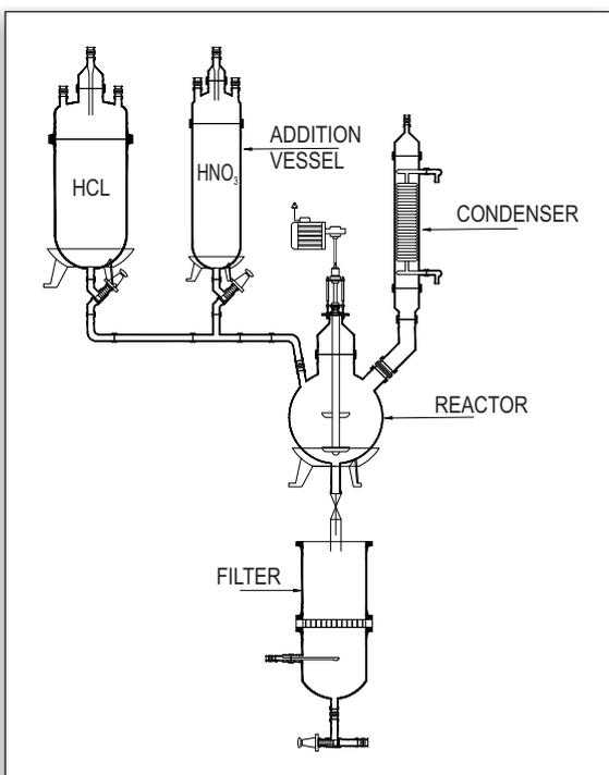
Borosilicate glass is inert to almost all materials. Due to which it is now widely used in Precious Metal Refining Industry. Borosilicate Glass is the only material which doesn't absorb precious metals. Its transparency allows ease of visualization & smooth surface allows ease of cleaning.
