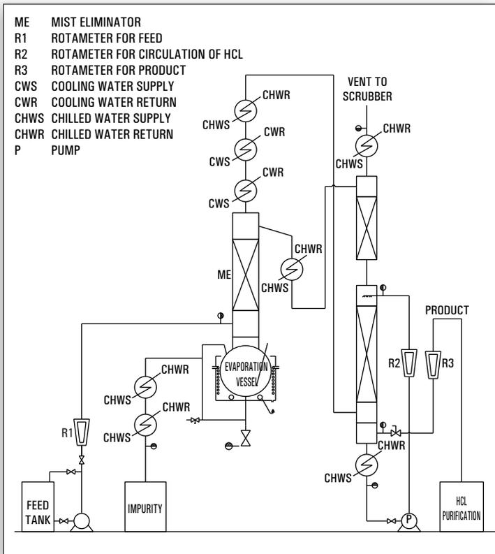
Commercial Grade Acid (30% HCL) is feed to the Reboiler through Flow meter. The feed will be heated in Re-Boiler by heating media to evaporate the 20-22% HCL. The 20-22% HCL+ Water Vapour generated will be condensed in Top Cooler with Cooling water & chilled water. The gas leaving the top will be of pure HCL gas will fed to the scrubber wherein it will be scrub further with condensed Azeotropic solution or with fresh process water to make ultrapure HCL.
