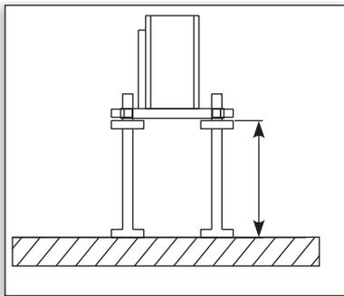
3. Put this assembly on the floor and prepare a rough surface for proper bonding of grouting.
