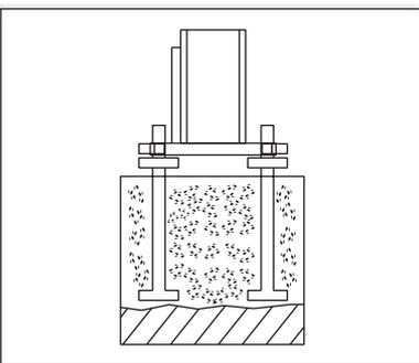
4. Make a concrete block over the bolts of about 200 x 200 mm upto the base of BASE i.e. 150mm high.
