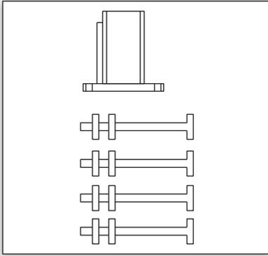
1. Take one Cast Iron BASE and four foundation Bolts, each with 2 nuts.
