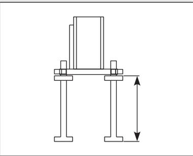
2. Fit the bolts in BASE so that base is raised upto 150mm from head of bolts.
