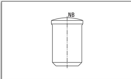
These are used to plug the open ends of galvanised tubes.
