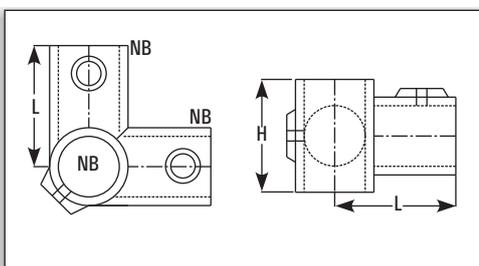
These are used to build frames on vertical tubes.
