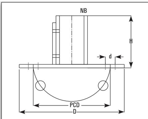
These are to be used with vertical tubes. Holes are provided for foundation.
