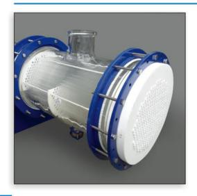
Permissible temperature range for both shell & tube sides -  $40^{\circ}$ C to  $150^{\circ}$ C. Maximum permissible temperature difference between shell & tube sides  $120^{\circ}$ C. All sizes & models are suitable for full vacuum on both side. Maximum limiting pressures are tabulated here below:
