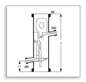
These reflux dividers are to be used with a electro-magnet and a timer. These have a swinging funnel machanism which is operated magnetically from outside to remove the condensate or to return the reflux. Through this, correct control of reflux-ratio is possible. Funnel remains at 100% reflux position while magnet is inactive.
