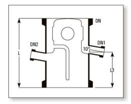
$\ensuremath{\mathsf{DN2}}$  is used for insertion of a thermometer pocket. A bellow is recommended on the distillate outlet  $\ensuremath{\mathsf{DN1}}.$
