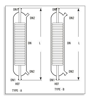
Product coolers are used for cooling of liquids, typically, for the cooling of distillates from the distillation columns.
