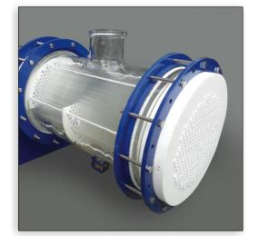
Permissible temperature range for both shell & tube sides -  $40^{\circ}$ C to  $150^{\circ}$ C. Maximum permissible temperature difference between shell & tube sides  $120^{\circ}$ C. All sizes & models are suitable for full vacuum on both side. Maximum limiting pressures are tabulated here below:
