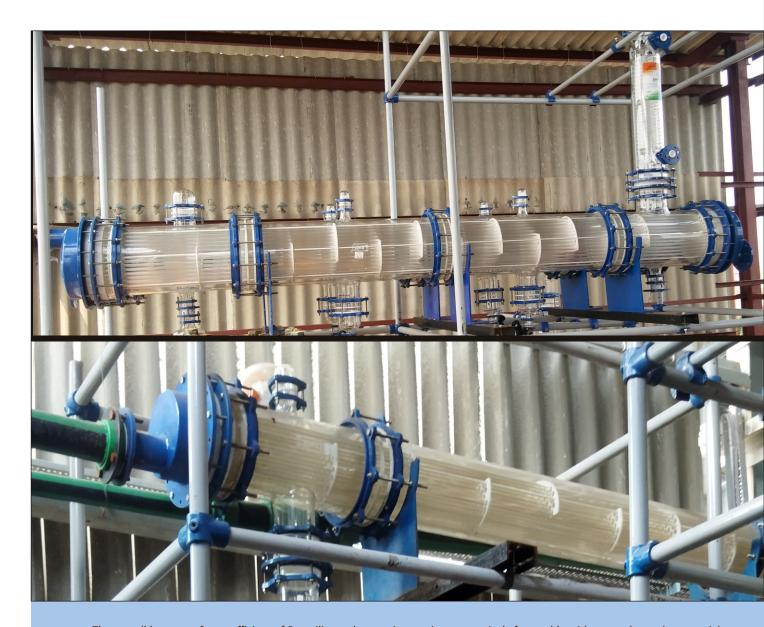
The overall heat transfer co-efficient of Borosilicate glass equipment is comparatively favourable with many alternative materials because of its smooth surface which improves the thermal coefficient & reduce the tendency of fouling.
