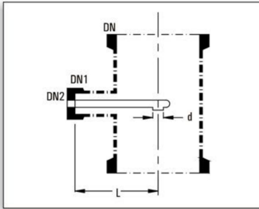
Feed pipe directs the process fluid to the centre of the column.
