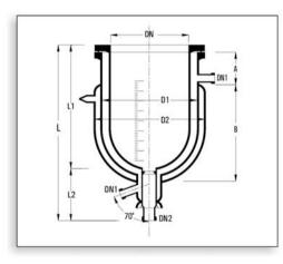
Goel is presenting Flexi (Detachable) "Transparent Double Jacketed Vessel" to maintain the leading position in industry by way of developing indigenously newer products with higher value towards their Mission and to cater the customer via innovation.
