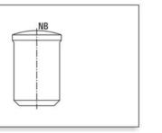
These are used to plug the open ends of galvanised tubes.
