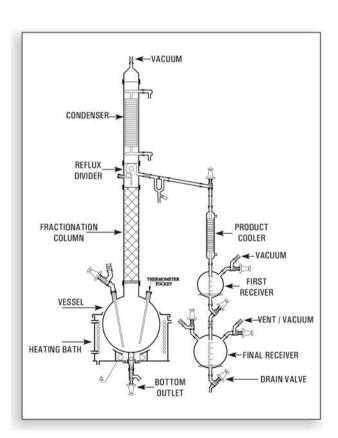
This is essentially a compact batch-type fractional distillation unit in which the reboiler consists of a vessel mounted in a heating bath and with a packed column above. The vapours from top is condensed and can be refluxed as per requirement.
