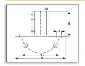
These are to be used with vertical tubes. Holes are provided for foundation.
