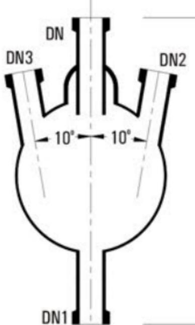
Receivers are provided with builtin drip pipe. These are to be supported on a vessel holding ring.
